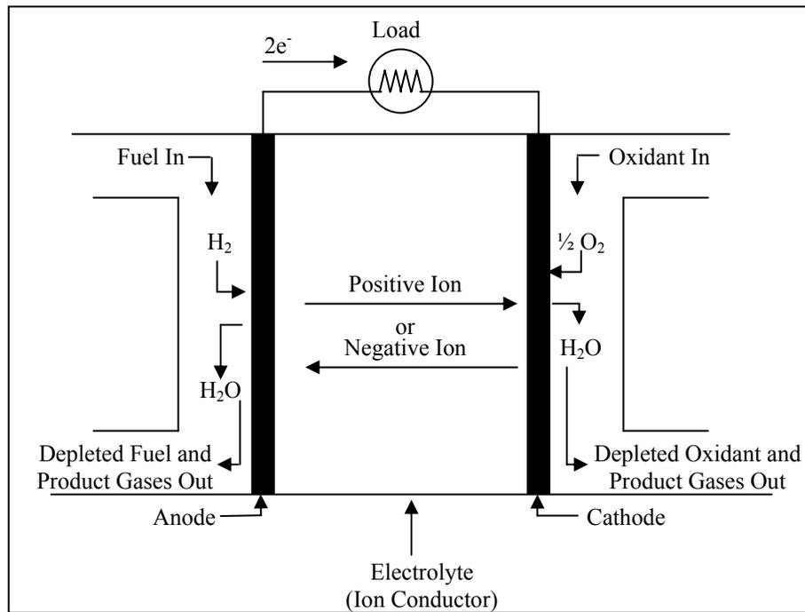
Figure 1 shows the basic cell configuration. The electrochemical reactions occurring within the cell are:
